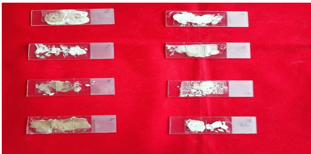
Fig 1: The synthesized silica particles from the surface of the Bacillus licheniformis .
