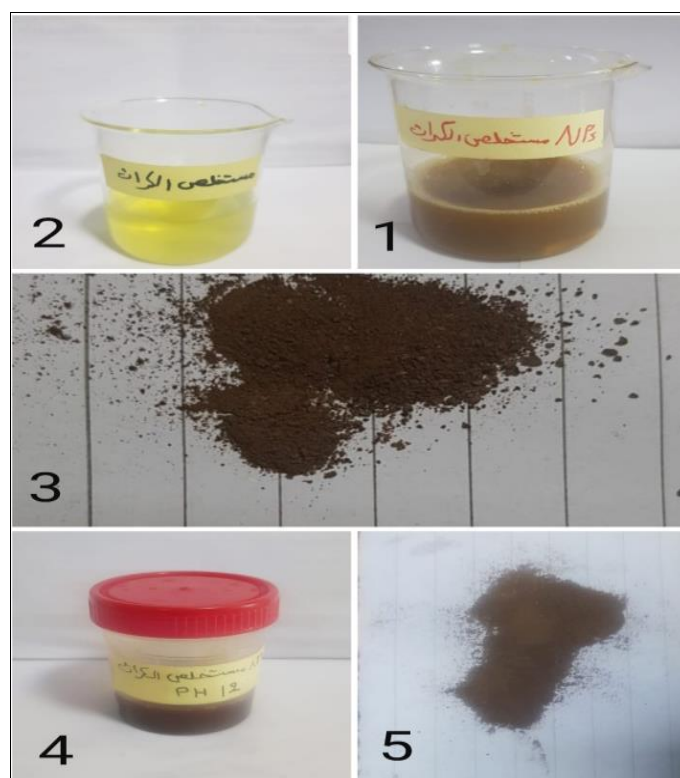
Fig 1: \alpha\text{-Fe}_2\text{O}_3 nanoparticle synthesis 1. Extract from leeks 2. IONPs at PH of 1.6 3. Pulverized at PH (1.6), 4- When PH (12), IONPs 5-powder at PH of 12
