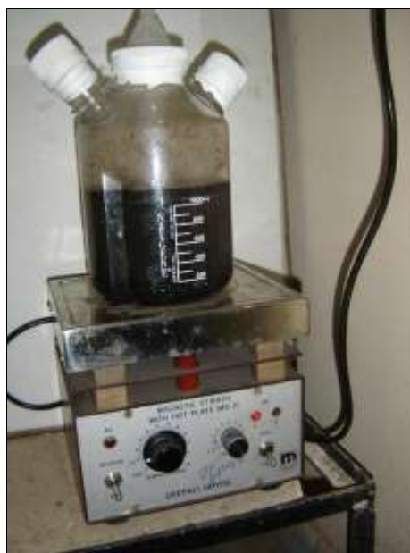
Fig 1: Anaerobic batch stirred tank Reactor
